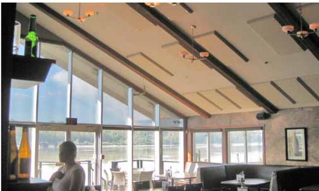
*Kingfishers pub in Maple Ridge, BC provides a beautiful view for customers but the glass wall and high vaulted ceiling contributed to long echos and poor intelligibility. Broadway acoustic panels installed on the ceiling retain the esthetic but fix the sound issues.*
