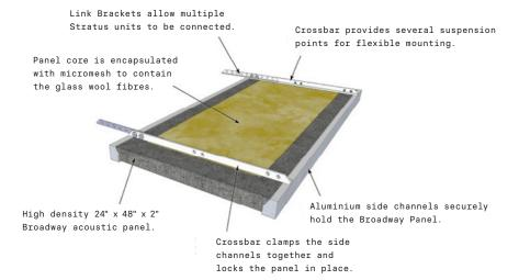
The Primacoustic Stratus is an acoustic cloud system designed to create large acoustic ceilings by linking multiple units together with a rigid frame.
