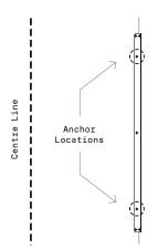
Hold the right crossbar up to the pencil line and mark the locations for the anchors.
