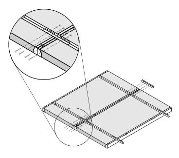
As with single clouds, ceiling anchors should be installed directly above the mounting points on the clouds. The diagram below shows the spacing of the mount points.
