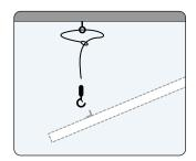
With the help of another person, lift one end of the Stratus or array up and clip the SlipNot hooks through the holes in the crossbar (single cloud suspension) or the link bracket (linked cloud suspension).
