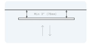
Fine-tune the lengths of the cable by pressing on the center sleeve of the anchor to release the cable. For the best acoustic performance, maintain a minimum of 3" (76mm) between cloud and ceiling.
