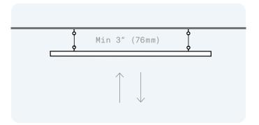
Fine-tune the lengths of the cable by pressing on the center sleeve of the anchor to release the cable. For the best acoustic performance, maintain a minimum of 3" (76mm) between cloud and ceiling.
