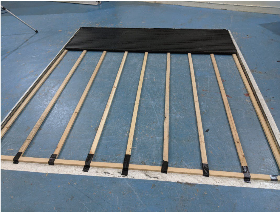
Figure 2 – Specimen partially installed over wood furring strips
