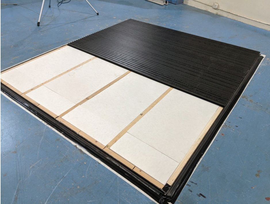
Figure 3 – ECOScapes panels partially installed over wood furring and TELAFILL panels
