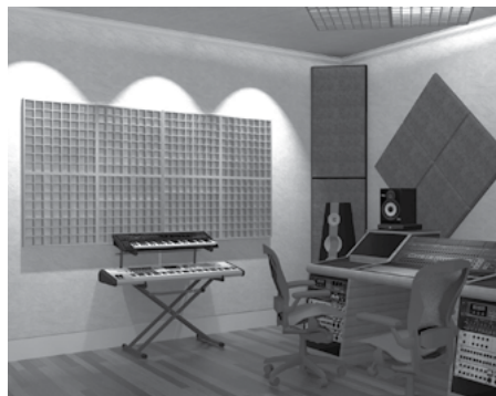
Eight Radiator diffusers are bolted together and hung on the wall to create ambiance in the studio.
