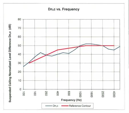
Dn,c = Normalized Ceiling Attenuation, dB Δ Dn,c = Uncertainty for 95% Confidence Level
